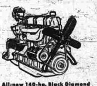
All-new 140-hp. Black Diamond economical sustained-power per-formance. Has new dual-barrel carburetor, new manifolding, 7.0-1 compression ratio—new low-friction design with 3-ring controlled-expan-sion pistons—new 50° ramp camahaft for longer valve life—new solenoidtype over-running clutch starter-new 11-inch clutch with 15% more lining area, 25% less pedal pressure. Maximum engine torque: 234 lb-ft at 2600 spm.
